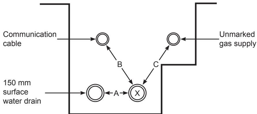
Give the minimum required separation distances between the services as indicated by A, B, and C.
